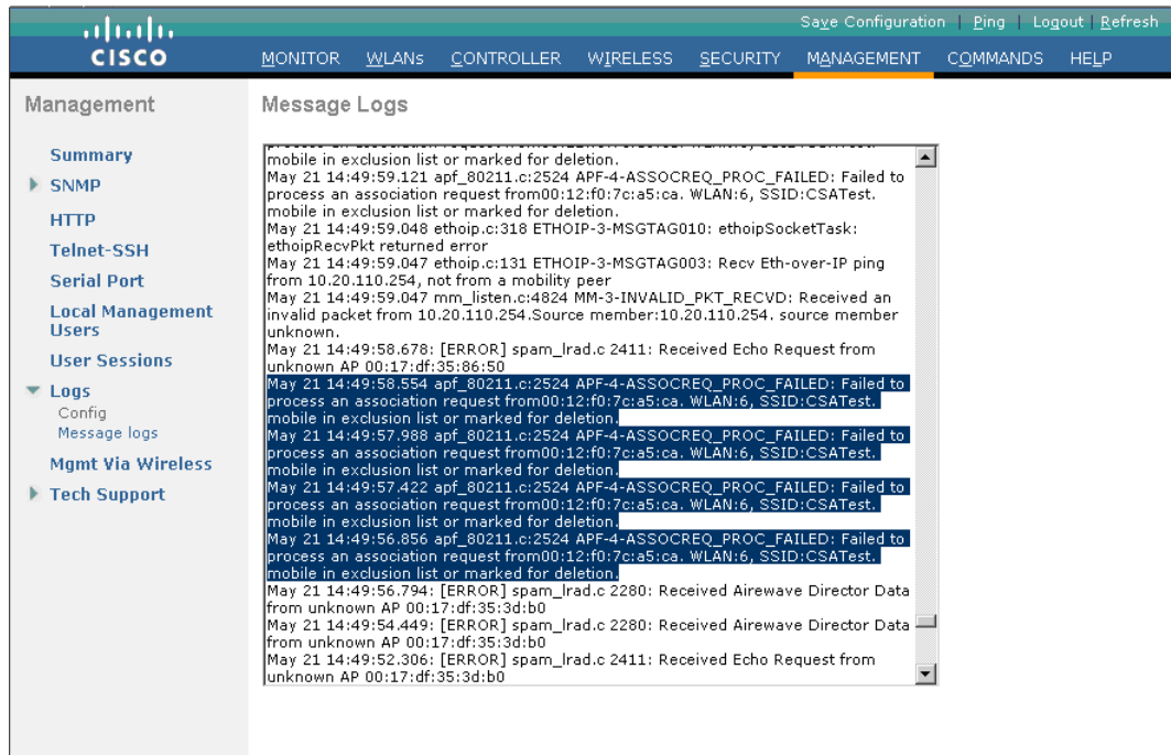
Figure 7-23 WLC Local Log Showing Multiple Attempts by a Blocked WLAN Client to Re-associate
