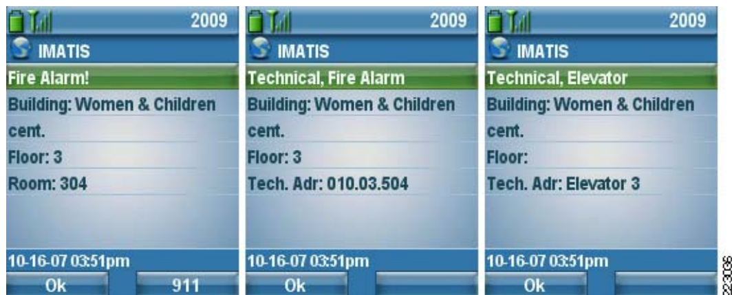
Figure 6-56 Alerts for Fire, Building, and Technical Problems
