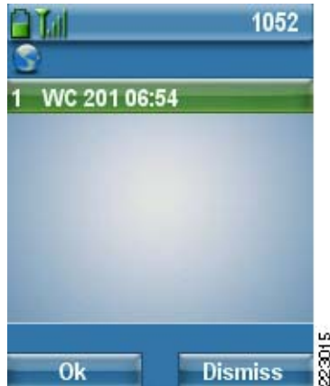
Figure 6-35 Alert Received by Nurse From Restroom Area
