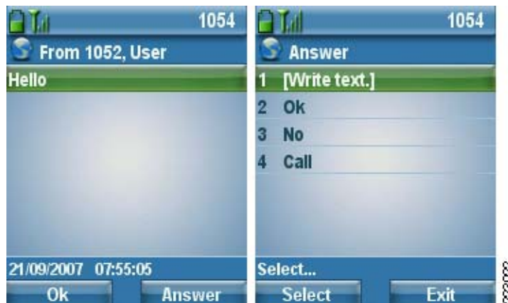
Figure 6-42 Example of User Receiving a Text Message and Options for Answering Message
