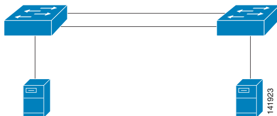
Figure 5-24 Logical EtherChannel Over EoMPLS
