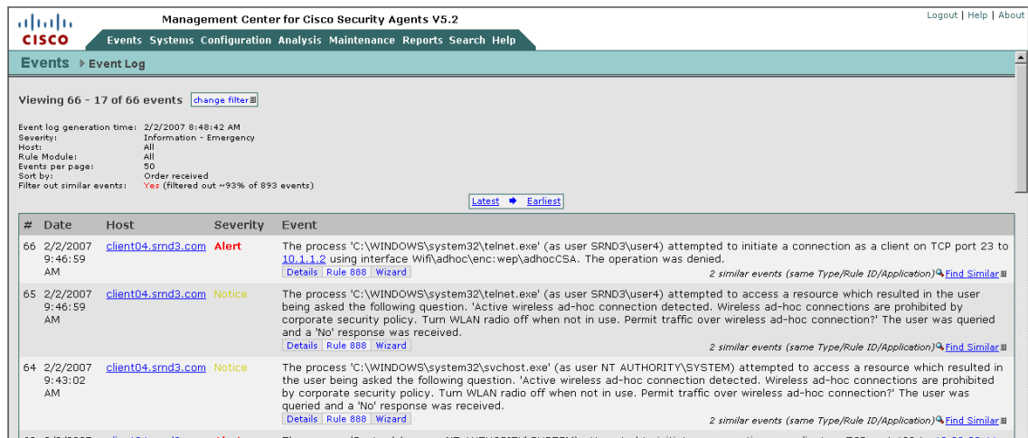
Figure 46 CSA MC Event Log Generated by Sample Customized Wireless Ad-hoc Rule
